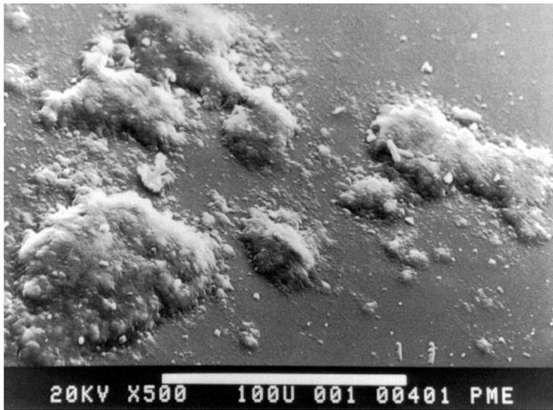
Figure 3. SEM image at 500X of paint deposit on glass.
