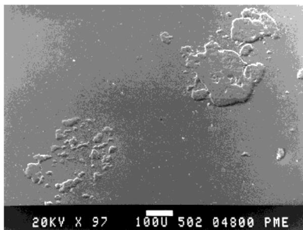
Figure 10. SEM image at 97X of sodium sulfate deposit on glass.
