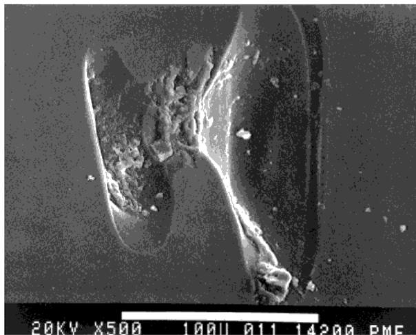
Figure 1. SEM image at 500X of bottom surface mechanical damage from glass debris on rollers.
