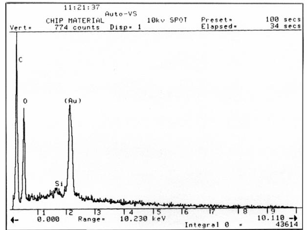
Figure 5. EDS spectrum of deposit shown in figure 4.
