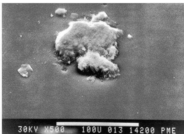
Figure 2. SEM image at 500X of bottom surface glass deposit.
