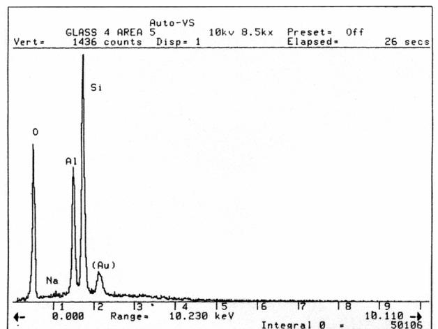
Figure 7. EDS spectrum of aluminosilicate refractory dust from fiber insulation on the glass as seen in figure 6.
