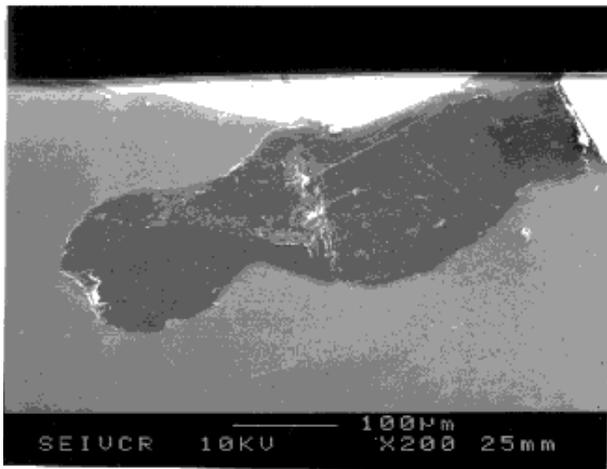
Figure 4. SEM image at 200X of glass defect from separation media that was not washed off of the glass prior to tempering.
