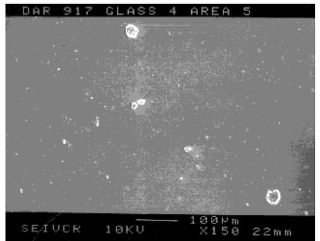
Figure 6. SEM image at 150X of refractory dust on glass.
