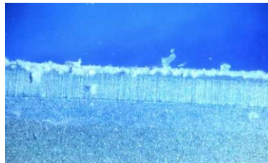
Figure 5 Debris may be observed on the edge of the scraper.
